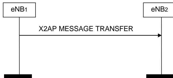
Figure 8.5.2-1: X2AP Message Transfer, successful operation
