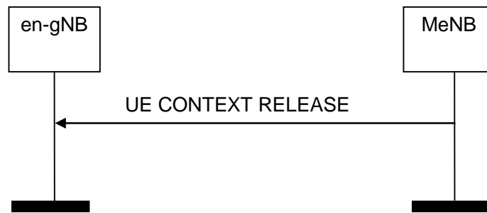
Figure 8.2.3.2-3: UE Context Release, successful operation for EN-DC
