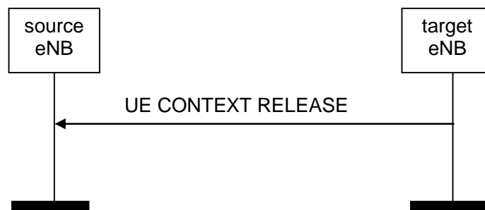
Figure 8.2.3.2-1: UE Context Release, successful operation for handover
