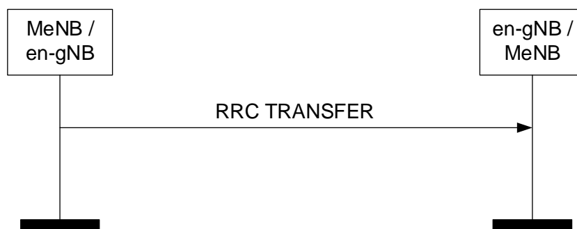
Figure 8.7.12.2-1: RRC Transfer procedure, successful operation.
