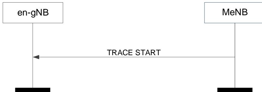
Figure 8.7.19.2-1: Trace Start, successful operation
