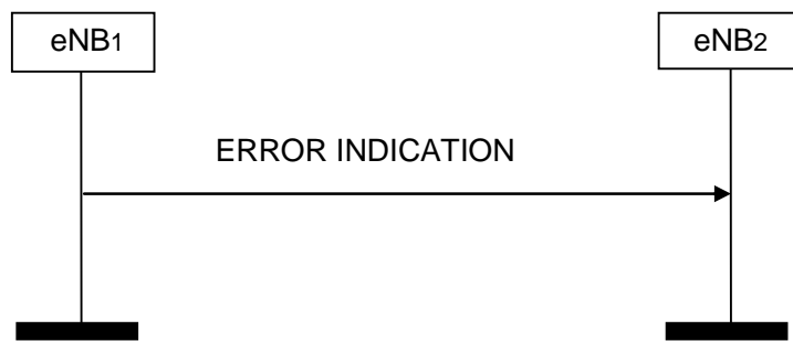
Figure 8.3.2.2-1: Error Indication, successful operation.
