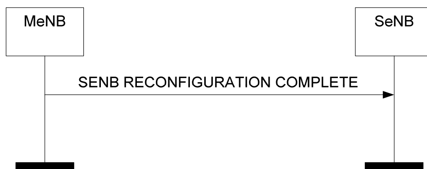
Figure 8.6.2.2-1: SeNB Reconfiguration Complete procedure, successful operation.
