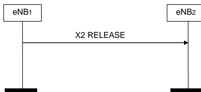
Figure 8.4.2-1: X2AP Release, successful operation
