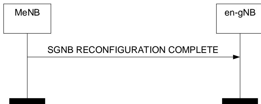
Figure 8.7.5.2-1: SgNB Reconfiguration Complete procedure, successful operation.
