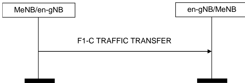
Figure 8.8.1.2-1: F1-C Traffic Transfer procedure, successful operation.
