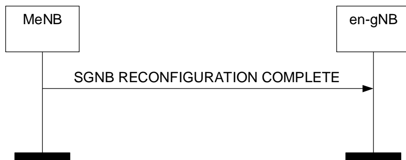
Figure 8.7.5.2-1: SgNB Reconfiguration Complete procedure, successful operation.
