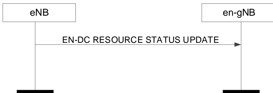
Figure 8.7.22.2-2: EN-DC Resource Status Reporting, successful operation - eNB-initiated
