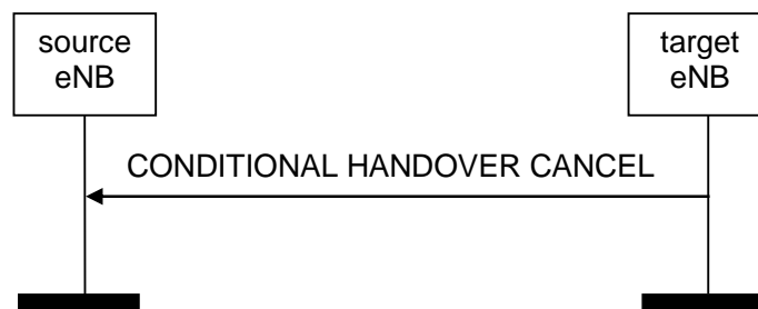
Figure 8.2.6.2-1: Conditional Handover Cancel, successful operation
