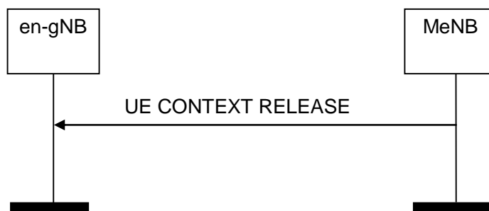
Figure 8.2.3.2-3: UE Context Release, successful operation for EN-DC
