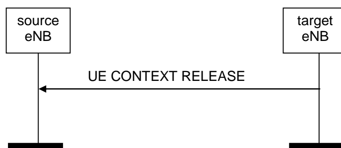
Figure 8.2.3.2-1: UE Context Release, successful operation for handover
