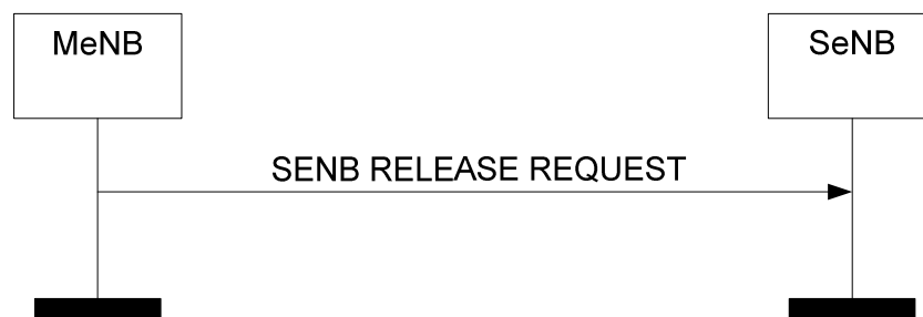
Figure 8.6.5.2-1: MeNB initiated SeNB Release, successful operation
