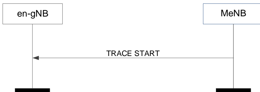
Figure 8.7.19.2-1: Trace Start, successful operation
