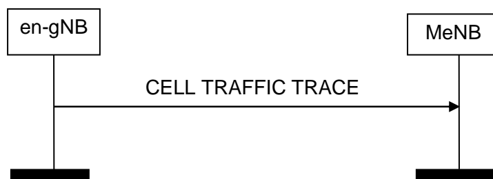
Figure 8.7.23.2-1: Cell Traffic Trace procedure. Successful operation.
