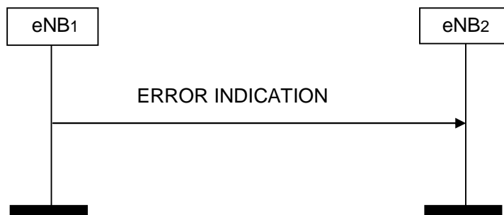
Figure 8.3.2.2-1: Error Indication, successful operation.
