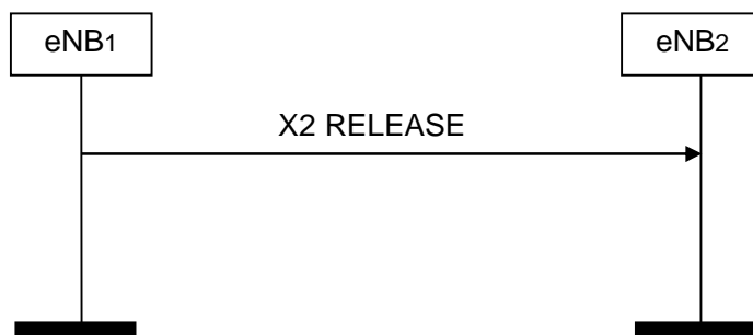
Figure 8.4.2-1: X2AP Release, successful operation
