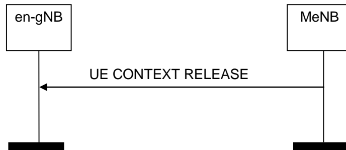
Figure 8.2.3.2-3: UE Context Release, successful operation for EN-DC
