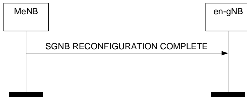
Figure 8.7.5.2-1: SgNB Reconfiguration Complete procedure, successful operation.
