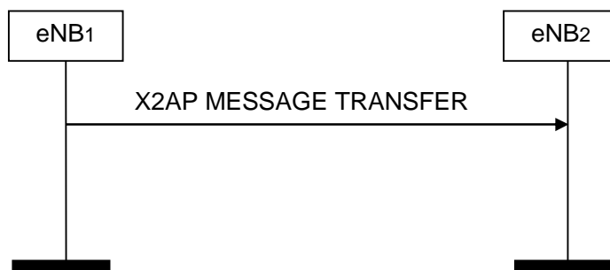
Figure 8.5.2-1: X2AP Message Transfer, successful operation
