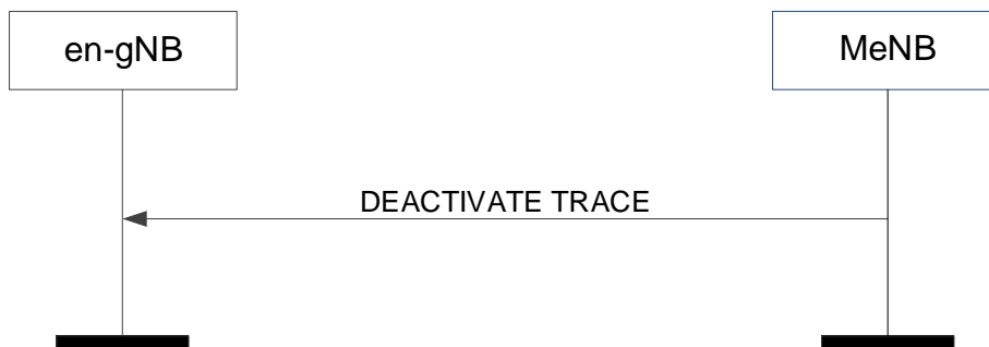
Figure 8.7.20.2-1: Deactivate Trace, successful operation
