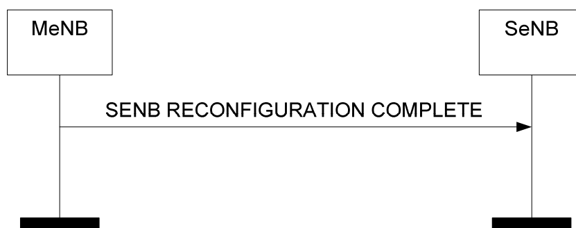
Figure 8.6.2.2-1: SeNB Reconfiguration Complete procedure, successful operation.
