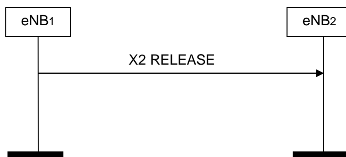
Figure 8.4.2-1: X2AP Release, successful operation
