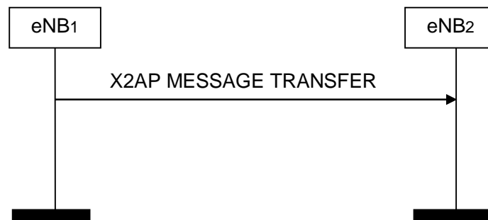
Figure 8.5.2-1: X2AP Message Transfer, successful operation
