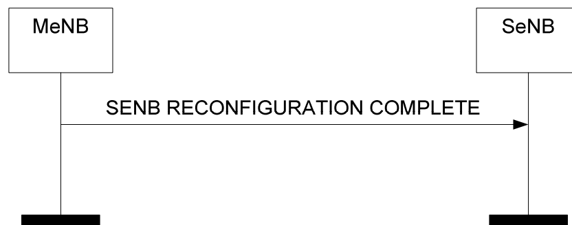
Figure 8.6.2.2-1: SeNB Reconfiguration Complete procedure, successful operation.
