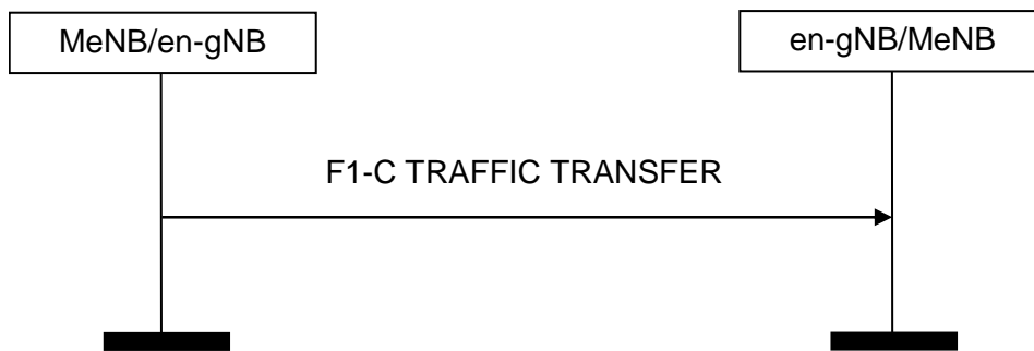
Figure 8.8.1.2-1: F1-C Traffic Transfer procedure, successful operation.
