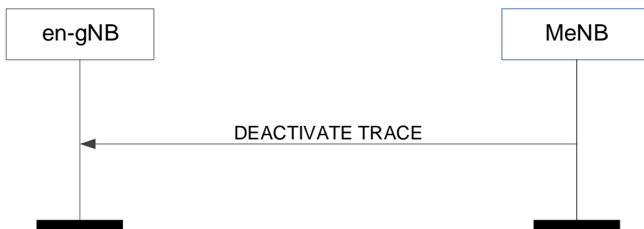
Figure 8.7.20.2-1: Deactivate Trace, successful operation
