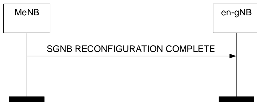
Figure 8.7.5.2-1: SgNB Reconfiguration Complete procedure, successful operation.
