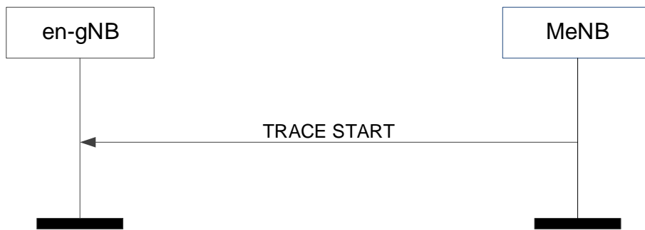
Figure 8.7.19.2-1: Trace Start, successful operation
