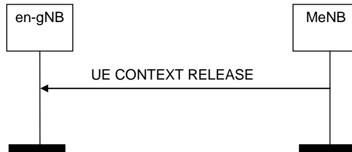
Figure 8.2.3.2-3: UE Context Release, successful operation for EN-DC
