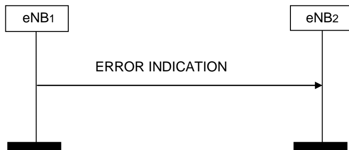
Figure 8.3.2.2-1: Error Indication, successful operation.
