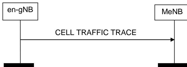
Figure 8.7.23.2-1: Cell Traffic Trace procedure. Successful operation.
