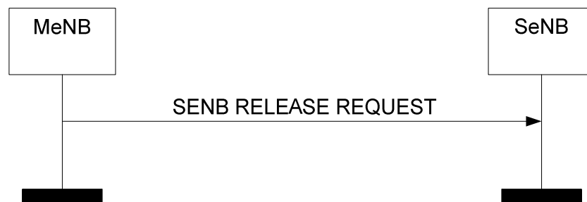
Figure 8.6.5.2-1: MeNB initiated SeNB Release, successful operation
