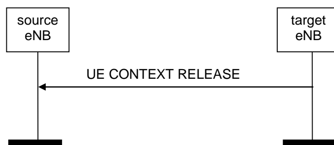
Figure 8.2.3.2-1: UE Context Release, successful operation for handover
