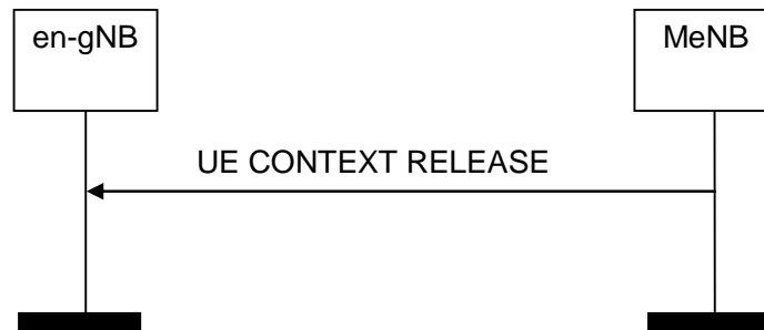
Figure 8.2.3.2-3: UE Context Release, successful operation for EN-DC
