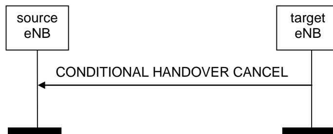
Figure 8.2.6.2-1: Conditional Handover Cancel, successful operation
