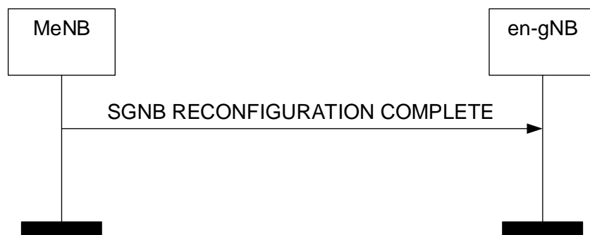
Figure 8.7.5.2-1: SgNB Reconfiguration Complete procedure, successful operation.
