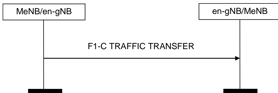
Figure 8.8.1.2-1: F1-C Traffic Transfer procedure, successful operation.
