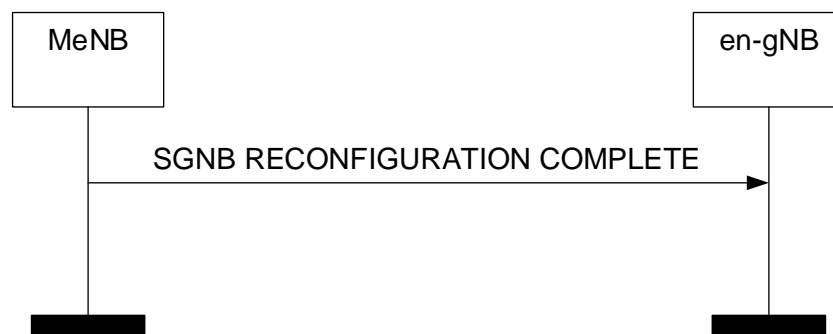
Figure 8.7.5.2-1: SgNB Reconfiguration Complete procedure, successful operation.
