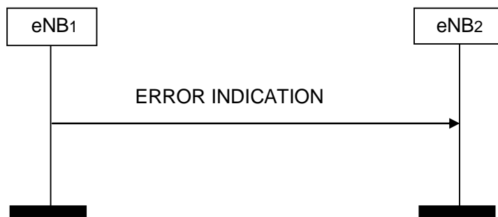
Figure 8.3.2.2-1: Error Indication, successful operation.
