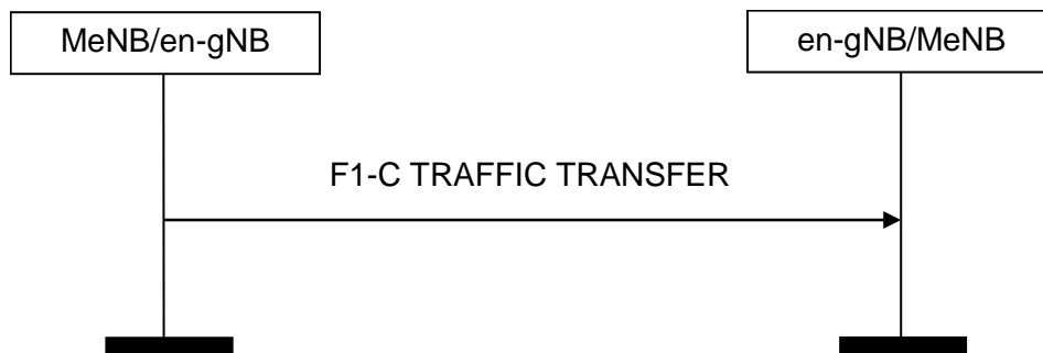
Figure 8.8.1.2-1: F1-C Traffic Transfer procedure, successful operation.
