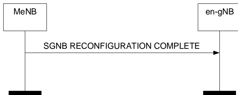
Figure 8.7.5.2-1: SgNB Reconfiguration Complete procedure, successful operation.
