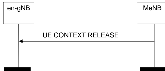
Figure 8.2.3.2-3: UE Context Release, successful operation for EN-DC
