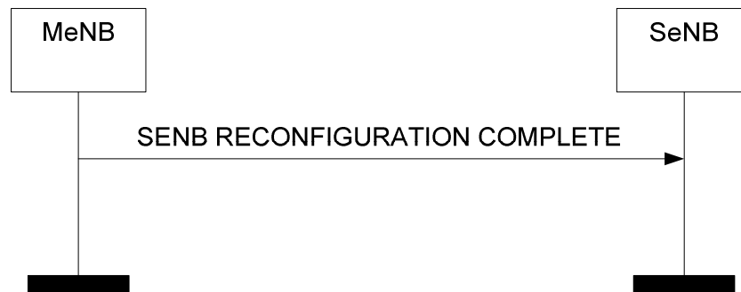
Figure 8.6.2.2-1: SeNB Reconfiguration Complete procedure, successful operation.
