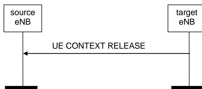
Figure 8.2.3.2-1: UE Context Release, successful operation for handover
