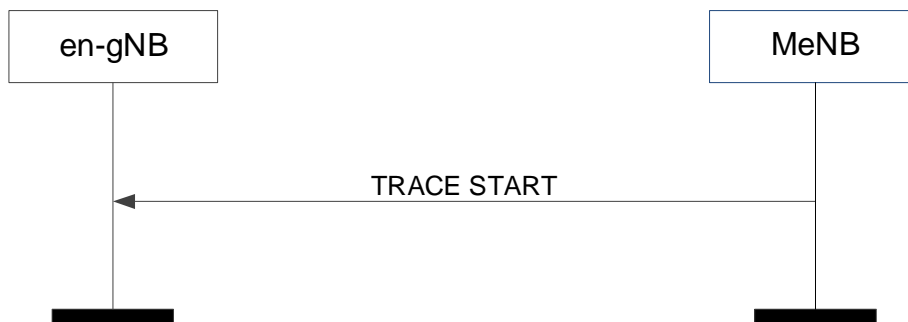
Figure 8.7.19.2-1: Trace Start, successful operation
