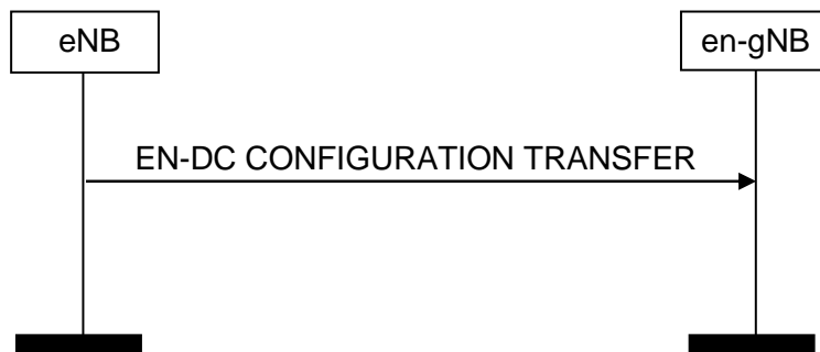
Figure 8.7.18.2-1: eNB initiated EN-DC Configuration Transfer, successful operation
