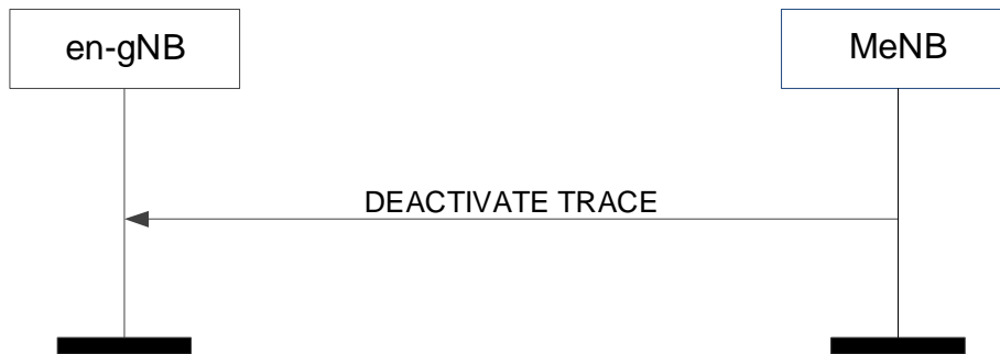
Figure 8.7.20.2-1: Deactivate Trace, successful operation
