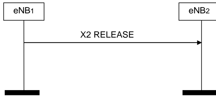
Figure 8.4.2-1: X2AP Release, successful operation
