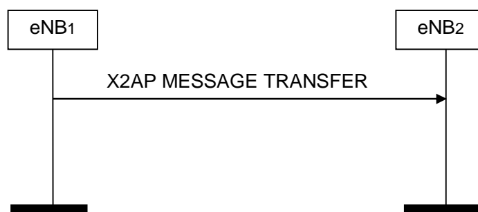
Figure 8.5.2-1: X2AP Message Transfer, successful operation
