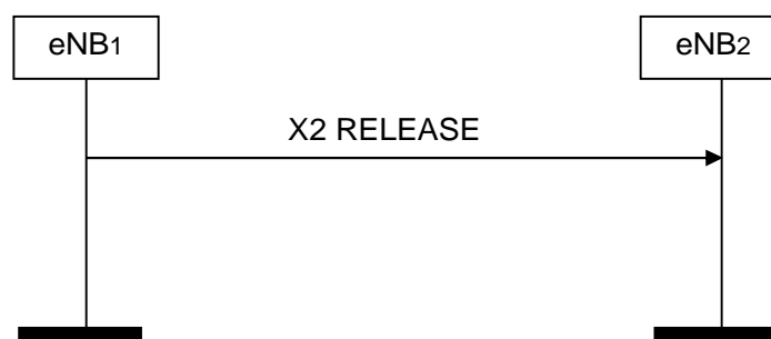
Figure 8.4.2-1: X2AP Release, successful operation
