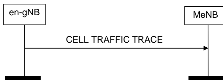
Figure 8.7.23.2-1: Cell Traffic Trace procedure. Successful operation.
