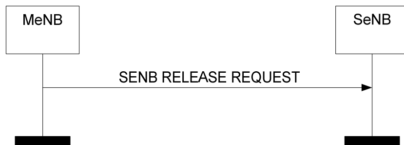
Figure 8.6.5.2-1: MeNB initiated SeNB Release, successful operation
