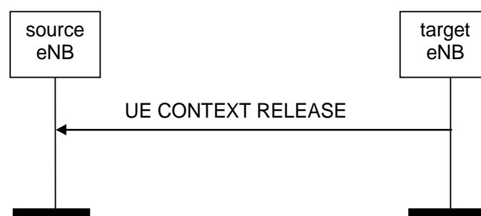
Figure 8.2.3.2-1: UE Context Release, successful operation for handover
