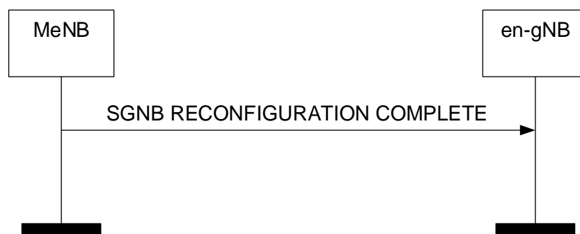
Figure 8.7.5.2-1: SgNB Reconfiguration Complete procedure, successful operation.
