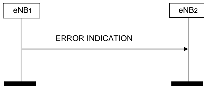
Figure 8.3.2.2-1: Error Indication, successful operation.
