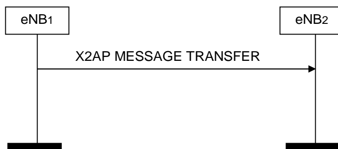
Figure 8.5.2-1: X2AP Message Transfer, successful operation
