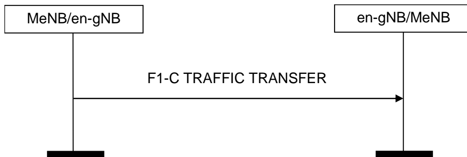
Figure 8.8.1.2-1: F1-C Traffic Transfer procedure, successful operation.
