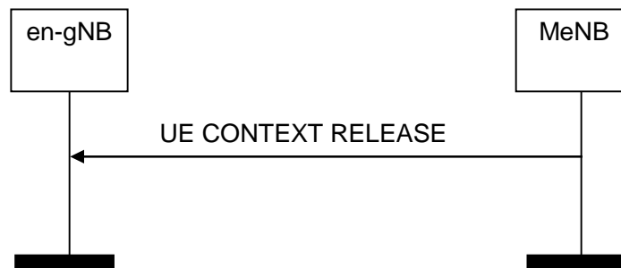
Figure 8.2.3.2-3: UE Context Release, successful operation for EN-DC
