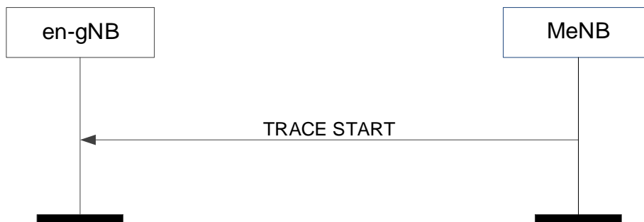
Figure 8.7.19.2-1: Trace Start, successful operation
