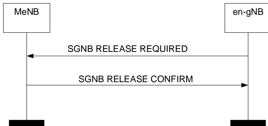
Figure 8.7.10.2-1: SgNB initiated SgNB Release, successful operation.
