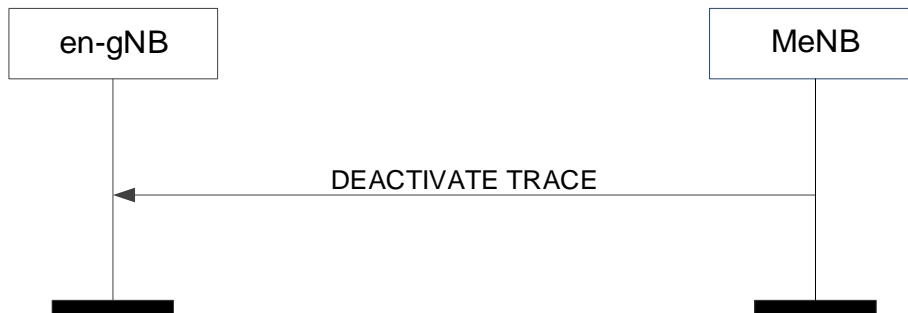
Figure 8.7.20.2-1: Deactivate Trace, successful operation
