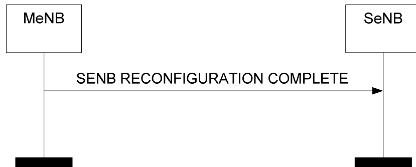
Figure 8.6.2.2-1: SeNB Reconfiguration Complete procedure, successful operation.
