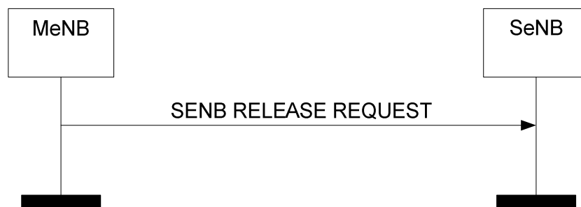
Figure 8.6.5.2-1: MeNB initiated SeNB Release, successful operation
