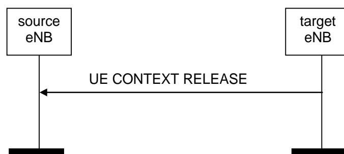
Figure 8.2.3.2-1: UE Context Release, successful operation for handover
