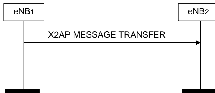
Figure 8.5.2-1: X2AP Message Transfer, successful operation
