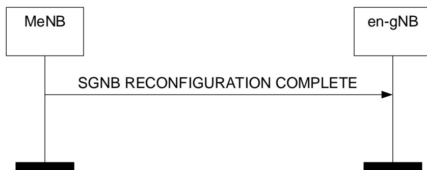
Figure 8.7.5.2-1: SgNB Reconfiguration Complete procedure, successful operation.
