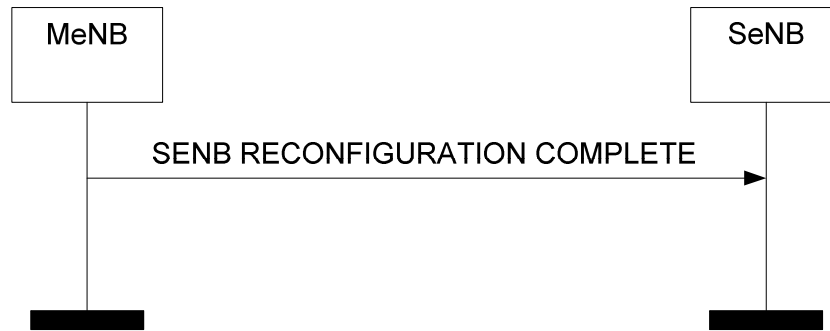
Figure 8.6.2.2-1: SeNB Reconfiguration Complete procedure, successful operation.
