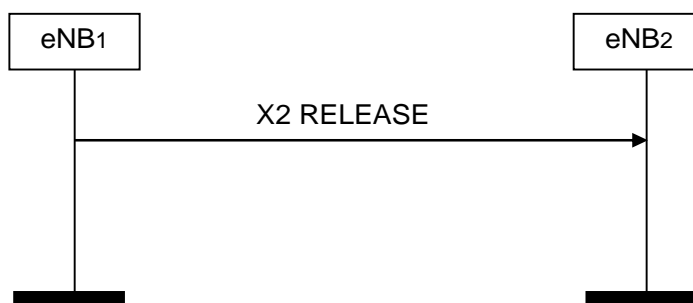
Figure 8.4.2-1: X2AP Release, successful operation
