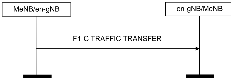
Figure 8.8.1.2-1: F1-C Traffic Transfer procedure, successful operation.
