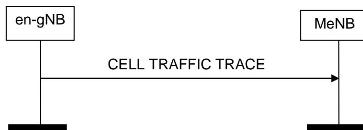
Figure 8.7.23.2-1: Cell Traffic Trace procedure. Successful operation.
