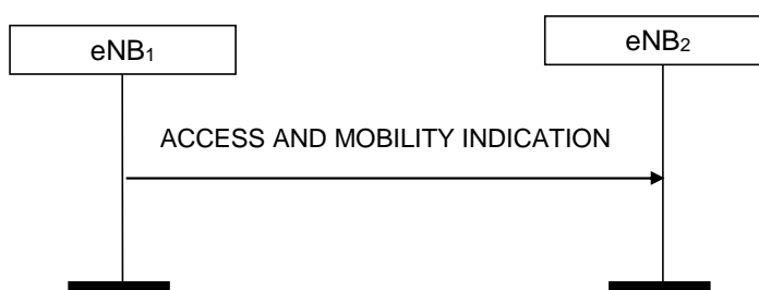
Figure 8.3.16.2-2: Access and Mobility Indication. Successful operation – eNB-initiated
