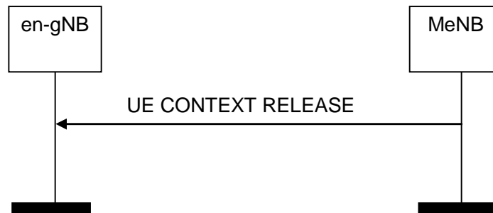
Figure 8.2.3.2-3: UE Context Release, successful operation for EN-DC
