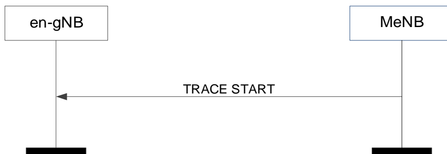
Figure 8.7.19.2-1: Trace Start, successful operation
