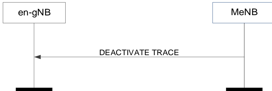
Figure 8.7.20.2-1: Deactivate Trace, successful operation
