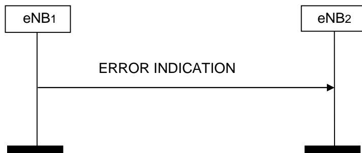
Figure 8.3.2.2-1: Error Indication, successful operation.
