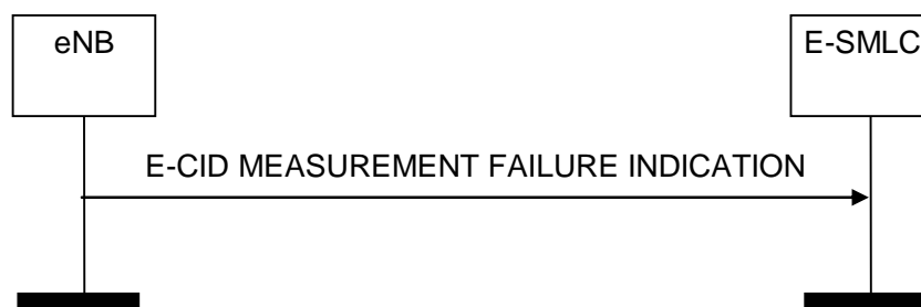
Figure 8.2.2.2-1: E-CID Measurement Failure Indication.
