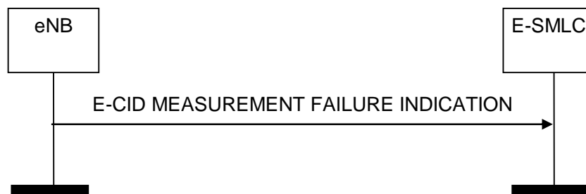
Figure 8.2.2.2-1: E-CID Measurement Failure Indication.
