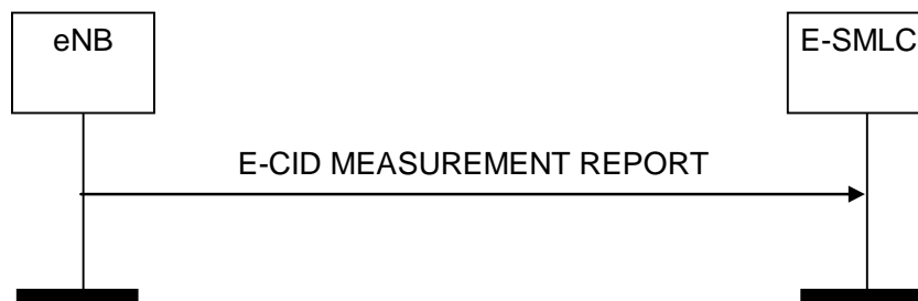
Figure 8.2.3.2-1: E-CID Measurement Report procedure, successful operation
