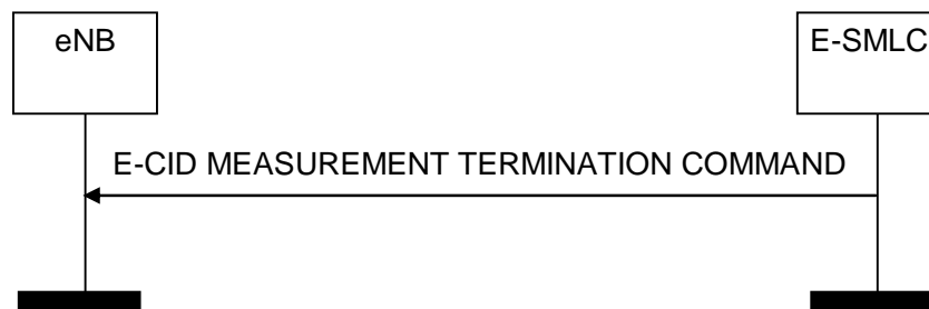
Figure 8.2.4.2-1: E-CID Measurement Termination procedure, successful operation
