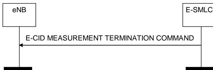
Figure 8.2.4.2-1: E-CID Measurement Termination procedure, successful operation
