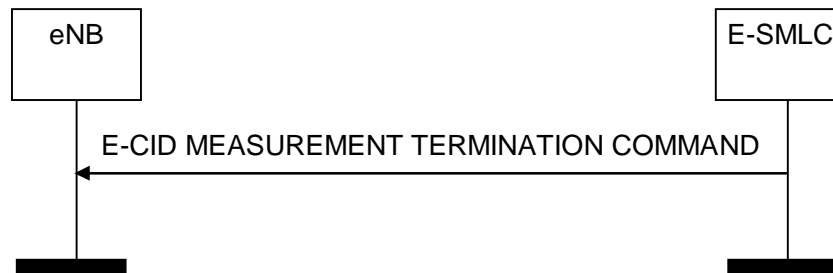
Figure 8.2.4.2-1: E-CID Measurement Termination procedure, successful operation
