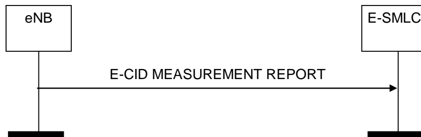
Figure 8.2.3.2-1: E-CID Measurement Report procedure, successful operation
