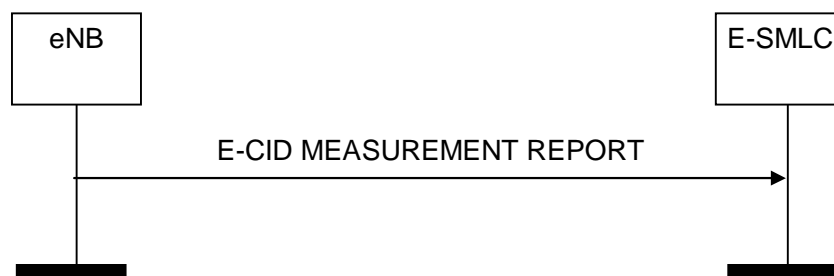
Figure 8.2.3.2-1: E-CID Measurement Report procedure, successful operation
