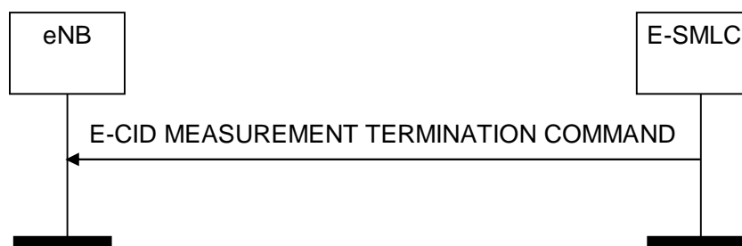
Figure 8.2.4.2-1: E-CID Measurement Termination procedure, successful operation
