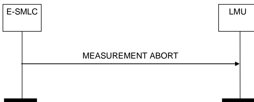
Figure 8.2.3.2.1: Measurement Abort Procedure: Successful Operation.
