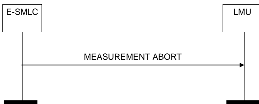
Figure 8.2.3.2.1: Measurement Abort Procedure: Successful Operation.
