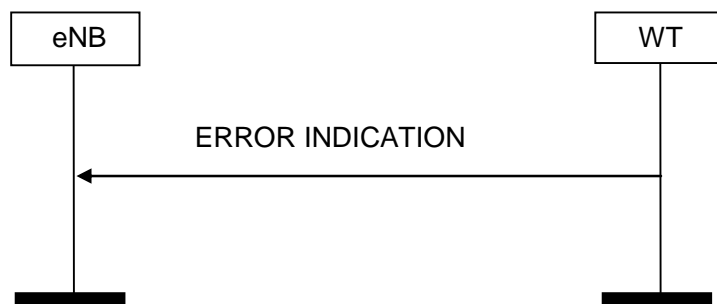
Figure 8.6.2-2: Error Indication procedure, WT originated. Successful operation.
