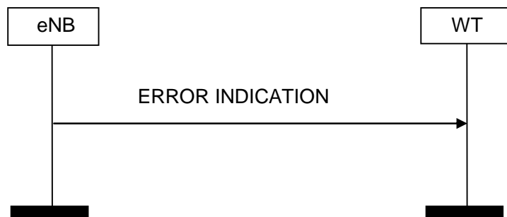
Figure 8.6.2-1: Error Indication procedure, eNB originated. Successful operation.
