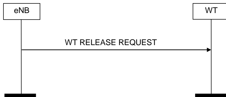
Figure 8.11.2-1: eNB initiated WT Release, successful operation
