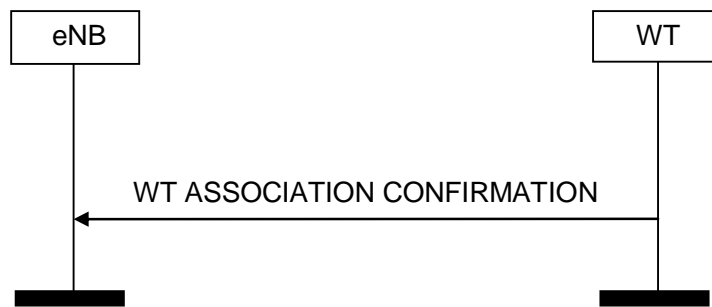
Figure 8.13.2-1: WT Association Confirm procedure, successful operation
