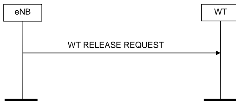
Figure 8.11.2-1: eNB initiated WT Release, successful operation
