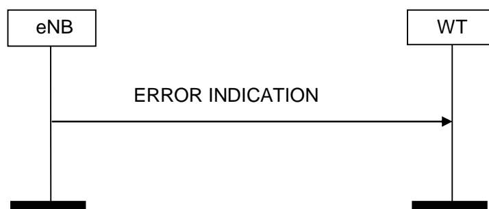
Figure 8.6.2-1: Error Indication procedure, eNB originated. Successful operation.
