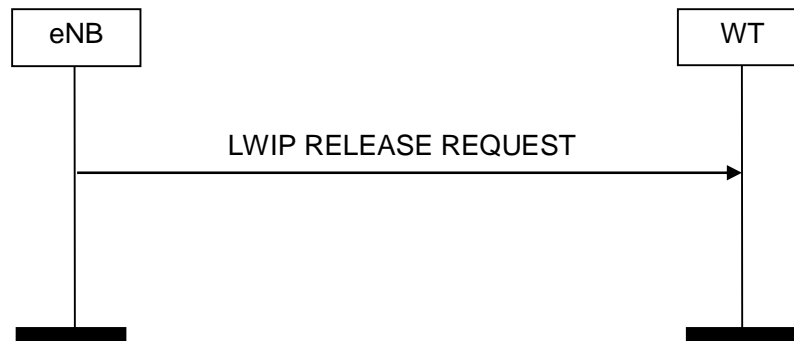
Figure 8.16.2-1: eNB initiated LWIP Release, successful operation
