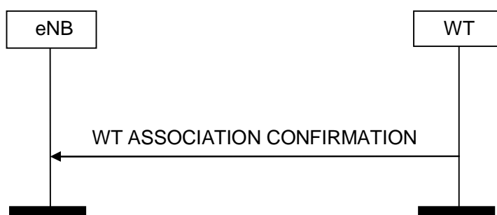
Figure 8.13.2-1: WT Association Confirm procedure, successful operation
