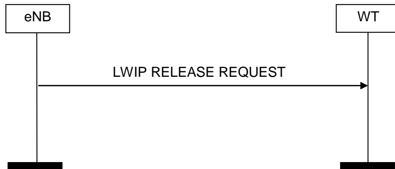
Figure 8.16.2-1: eNB initiated LWIP Release, successful operation
