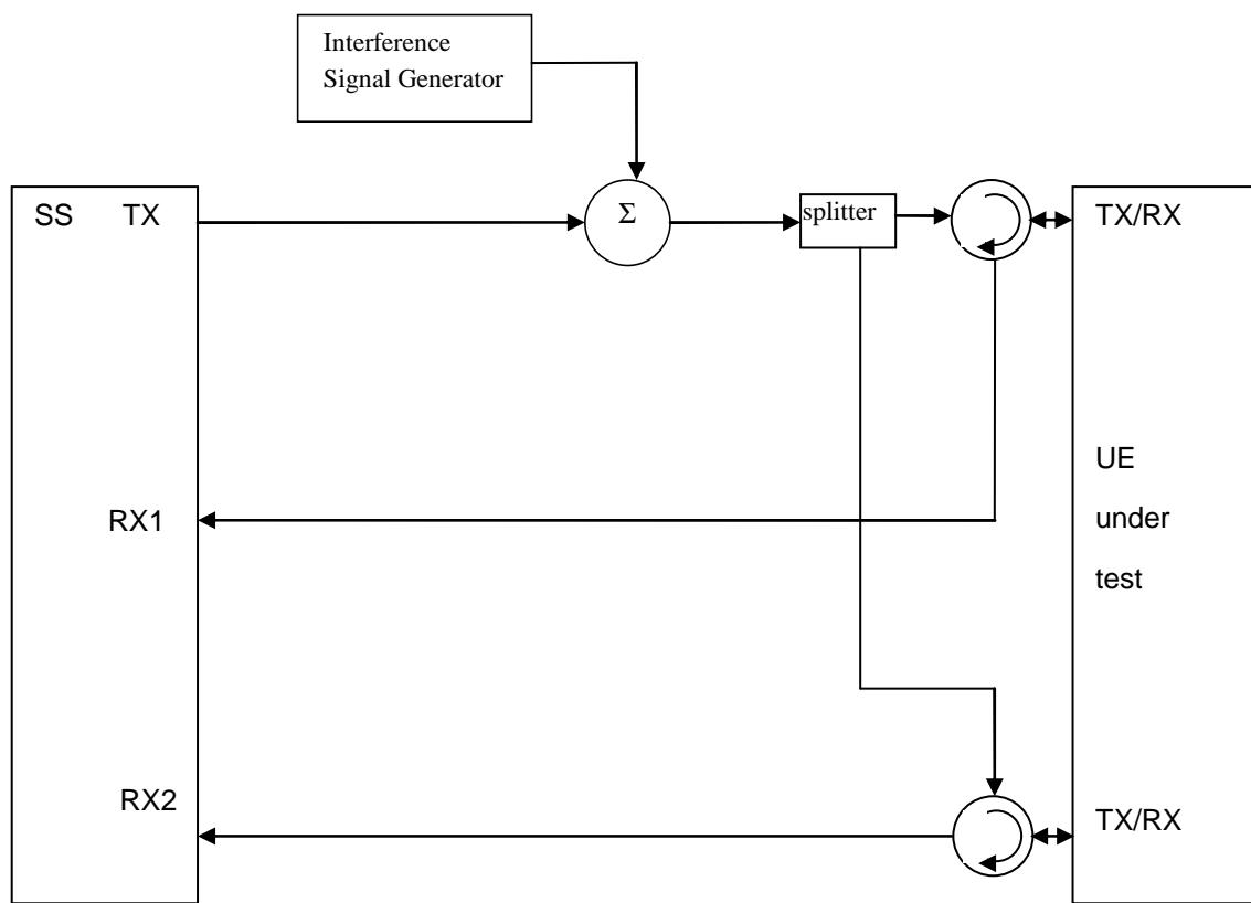
**Figure A.29: Connection for UL MIMO Receiver tests with E-UTRA-Interference**
