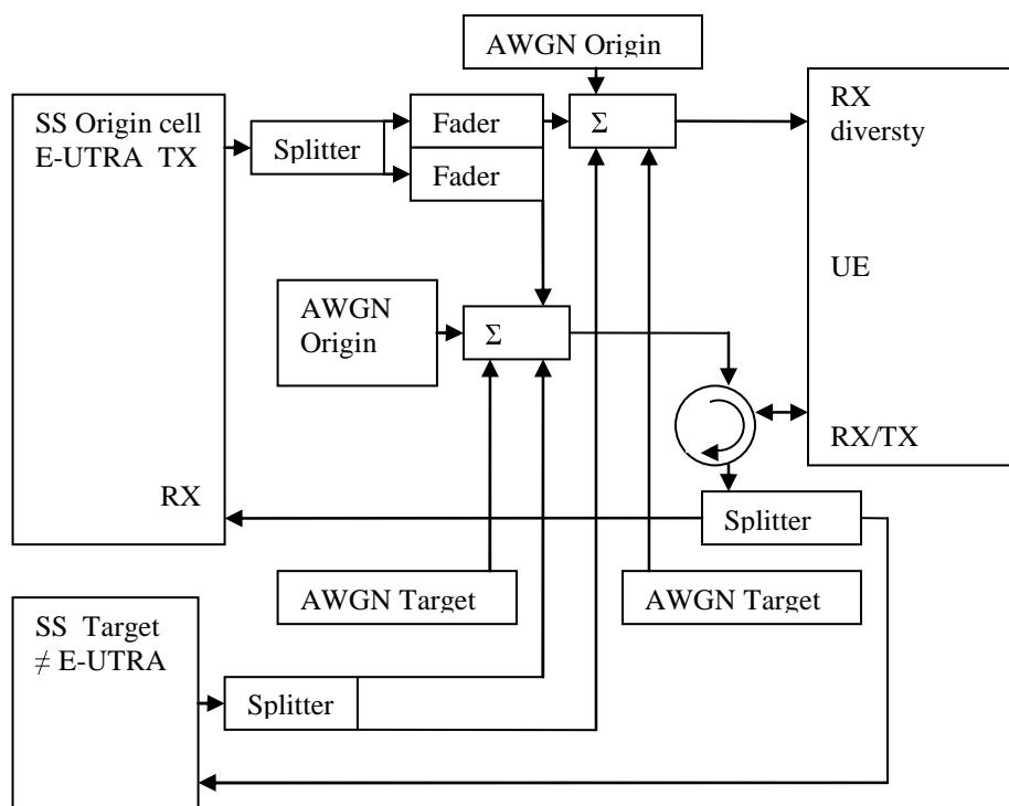
**Figure A.26: Connection for 2 cells. Origin (E-UTRAN, multipath fading) and target cell ( $\neq$  E-UTRAN, static) received with RX diversity**
