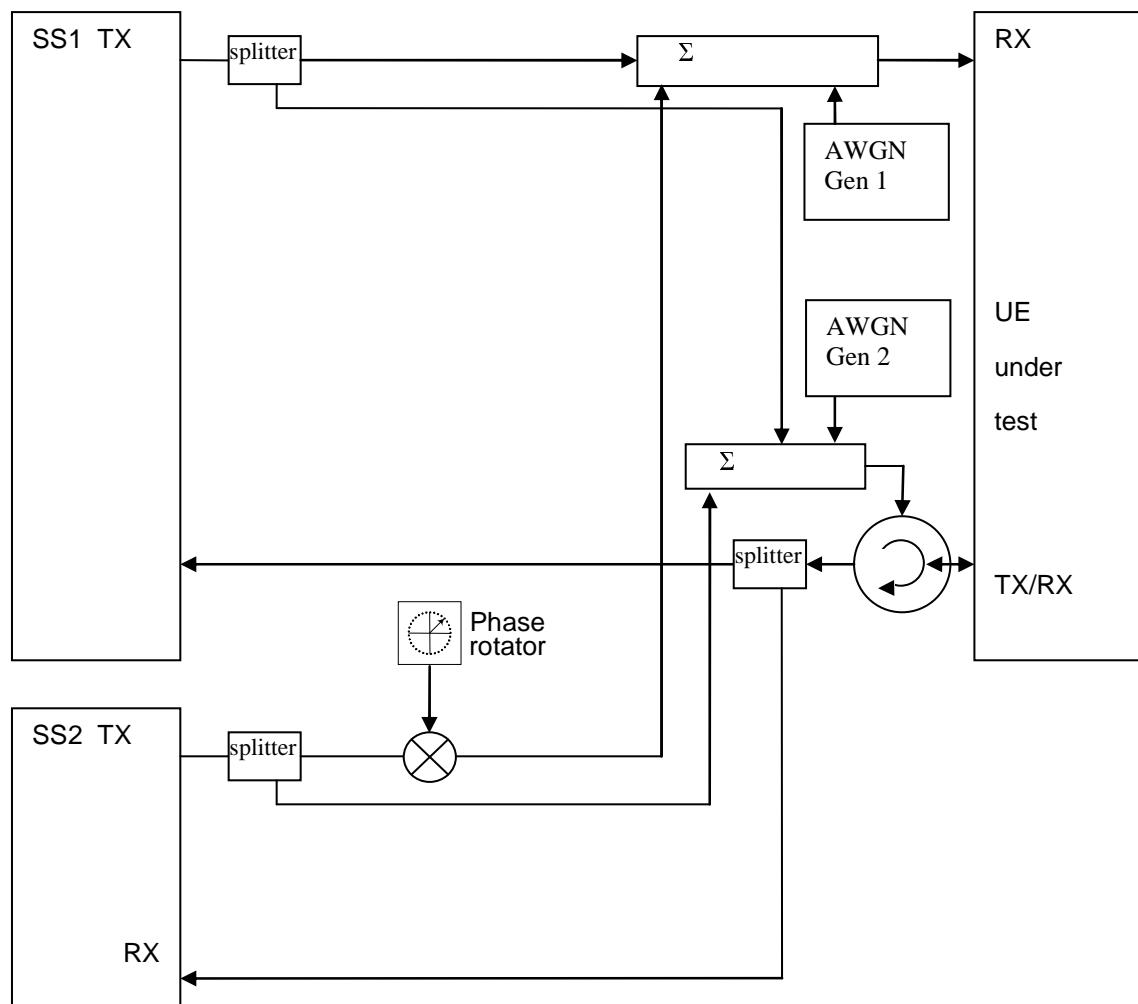
**Figure A.20: Connection for 2 cells with static propagation and receive diversity with phase rotator
