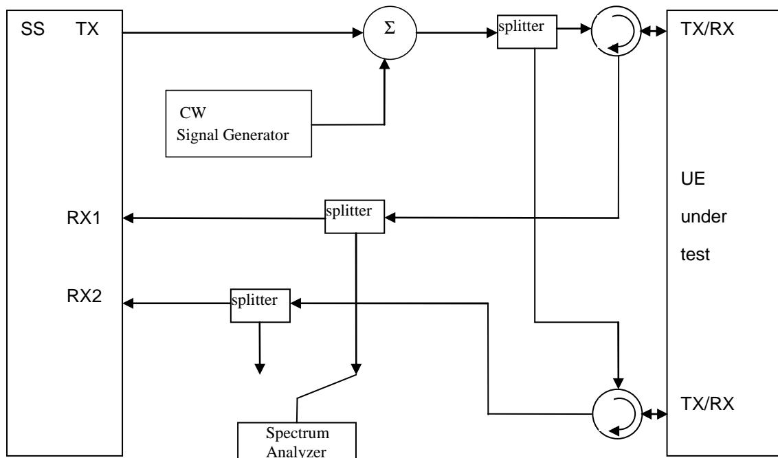
Figure A.39: Connection for Transmitter Intermodulation tests for UL-MIMO
