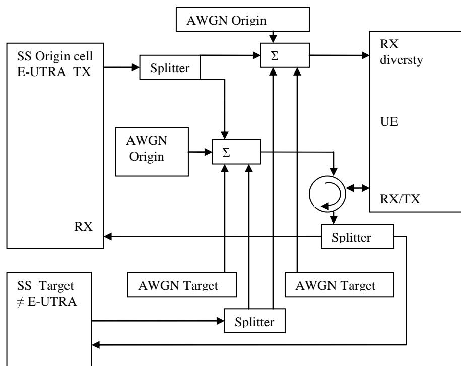
**Figure A.22: Connection for 2 cells with static propagation condition. Origin (E-UTRAN) and target cell (# E-UTRAN) received with RX diversity**
