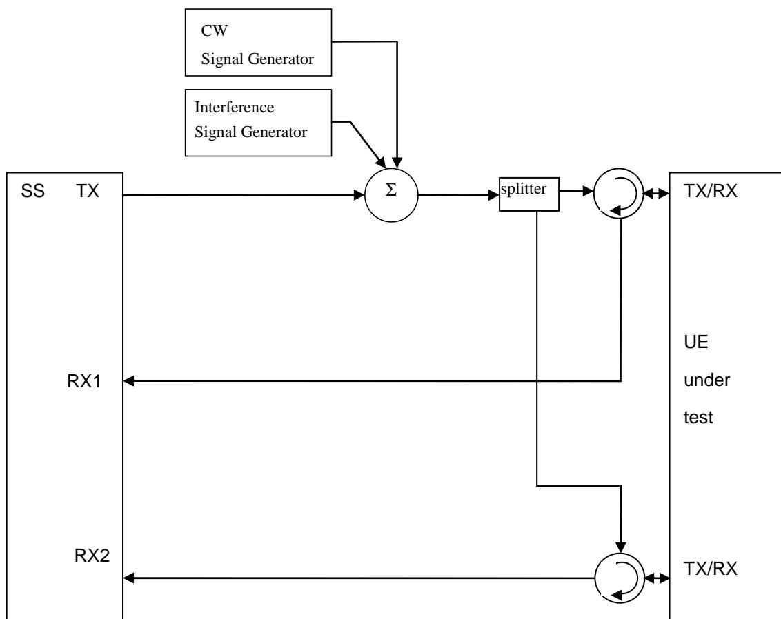
**Figure A.31: Connection for UL MIMO Receiver tests with both E-UTRA-Interference and additional CW signal**
