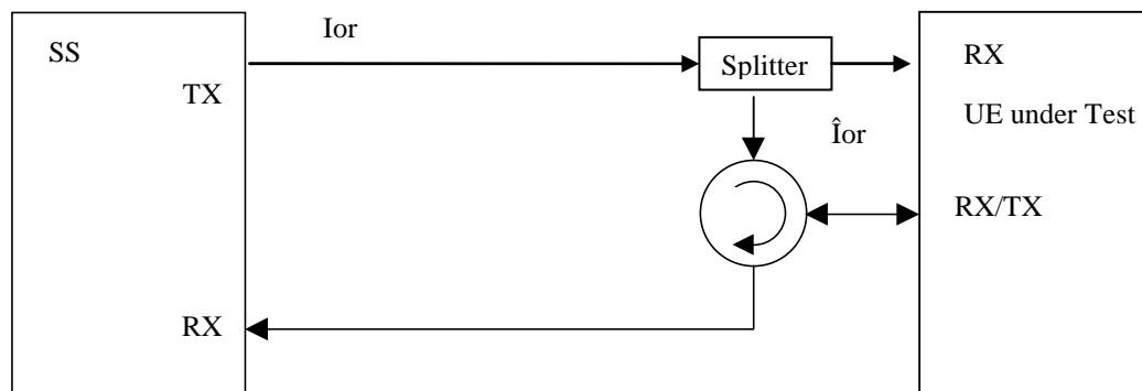
Figure A.3: Connection for basic single cell, RX and TX tests
