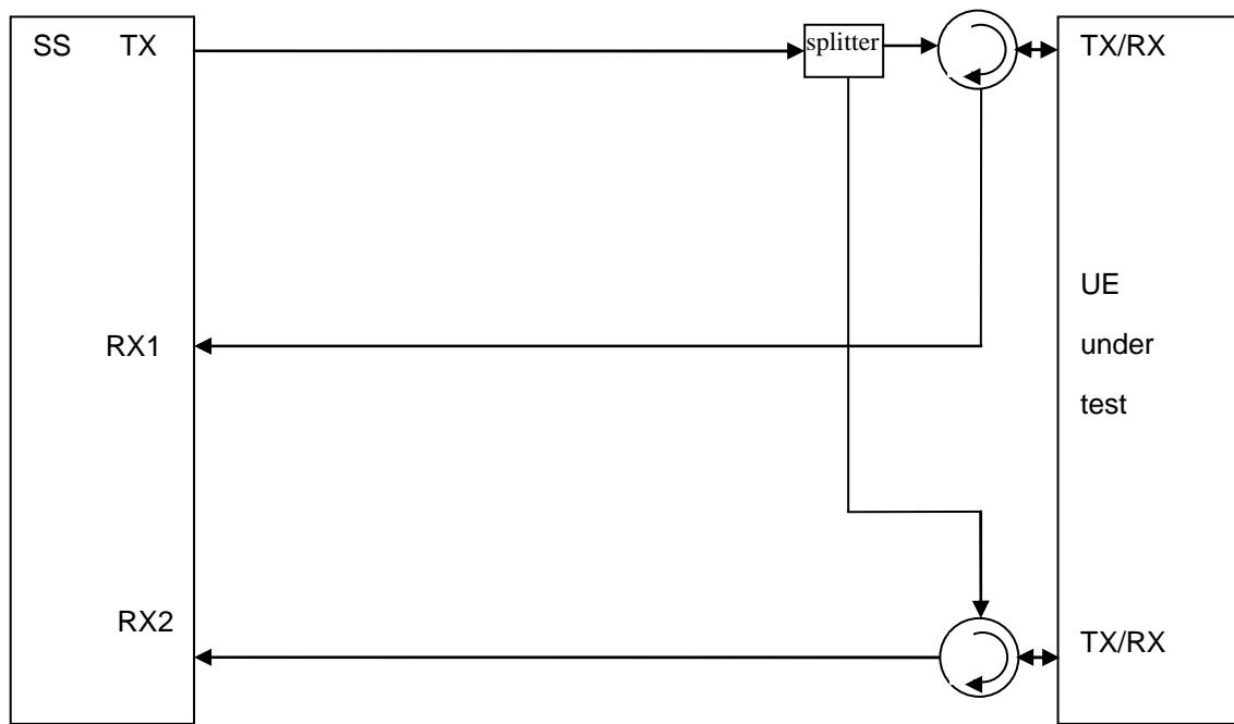
**Figure A.28: Connection for basic UL MIMO with receive diversity**
