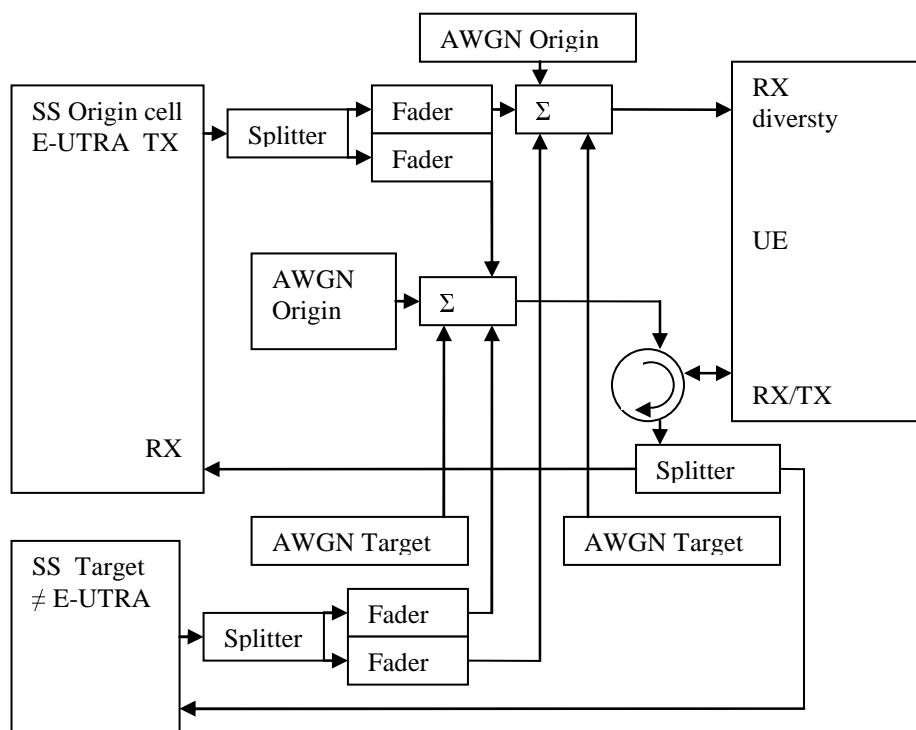
**Figure A.23: Connection for 2 cells with multipath fading propagation condition. Origin (E-UTRAN) and target cell ( $\neq$  E-UTRAN) received with RX diversity**
