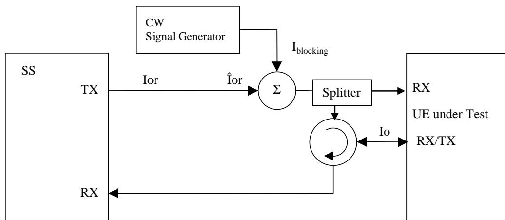
**Figure A.5: Connection for Receiver tests with CW interferer**
