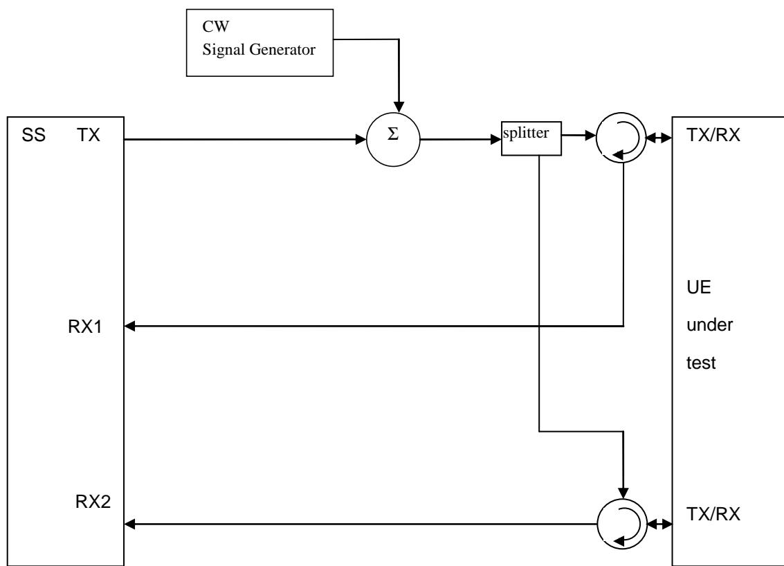
**Figure A.30: Connection for UL MIMO Receiver tests with CW Interference**
