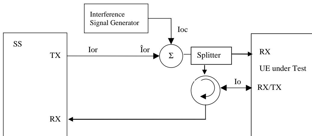
**Figure A.4: Connection for Receiver tests with E-UTRA-Interference**
