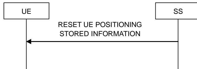
Figure 5.5.1-1: Reset UE Positioning Stored Information procedure
