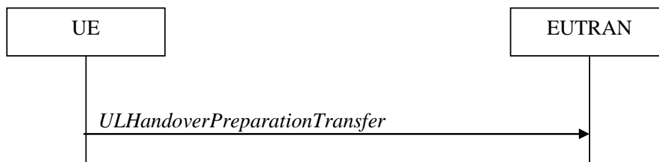
Figure 5.4.5.1-1: UL handover preparation transfer
