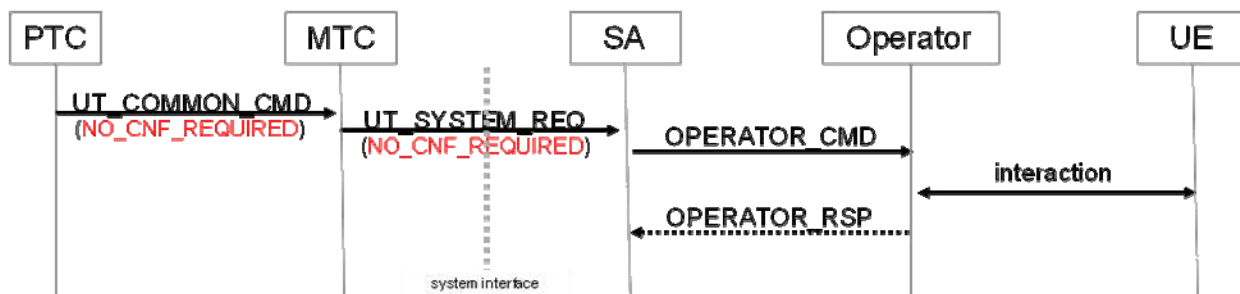
Figure E.1-2: No confirmation (manual intervention)
