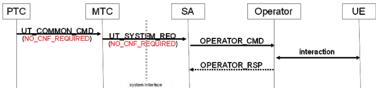
Figure E.1-2: No confirmation (manual intervention)
