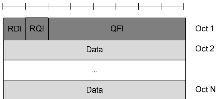
Figure 6.2.2.2-1: DL SDAP Data PDU format with SDAP header
