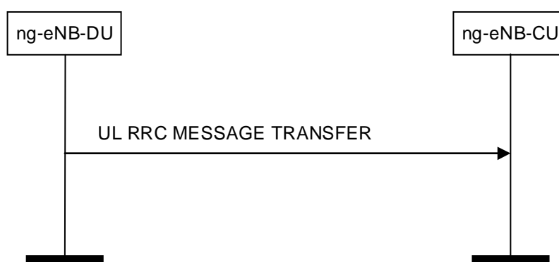
Figure 8.4.3.2-1: UL RRC Message Transfer procedure
