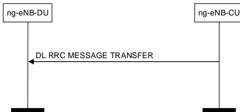
Figure 8.4.2.2-1: DL RRC Message Transfer procedure
