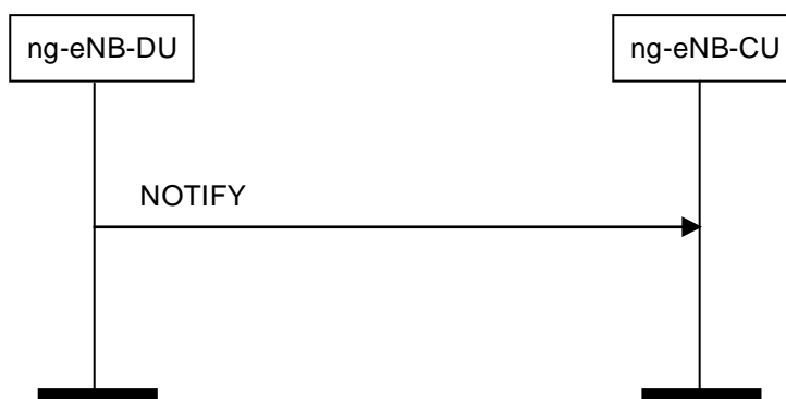
Figure 8.3.7.2-1: Notify procedure. Successful operation.
