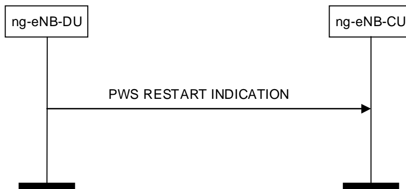
Figure 8.5.3.2-1: PWS restart indication
