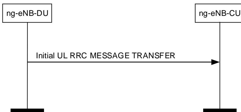
Figure 8.4.1.2-1: Initial UL RRC Message Transfer procedure
