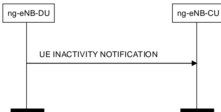
Figure 8.3.6.2-1: UE Inactivity Notification procedure.
