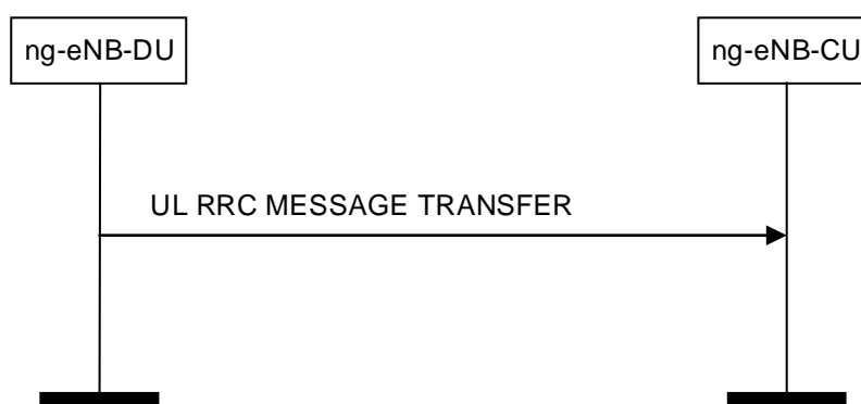
Figure 8.4.3.2-1: UL RRC Message Transfer procedure
