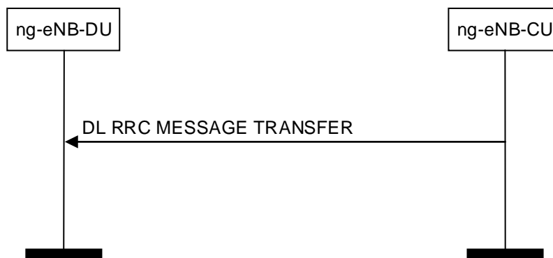
Figure 8.4.2.2-1: DL RRC Message Transfer procedure
