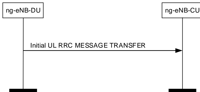
Figure 8.4.1.2-1: Initial UL RRC Message Transfer procedure
