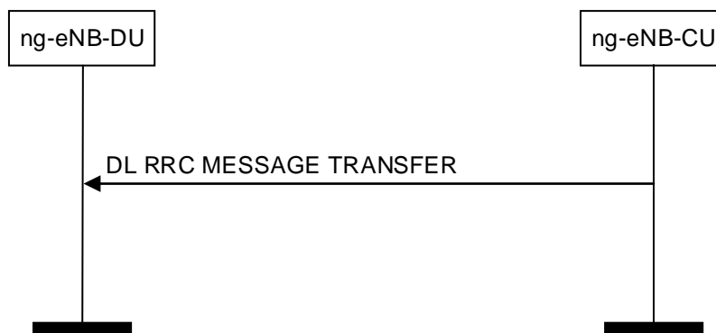
Figure 8.4.2.2-1: DL RRC Message Transfer procedure
