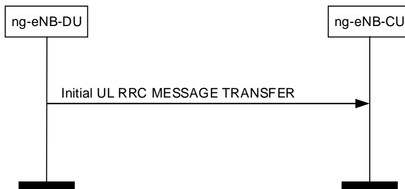
Figure 8.4.1.2-1: Initial UL RRC Message Transfer procedure
