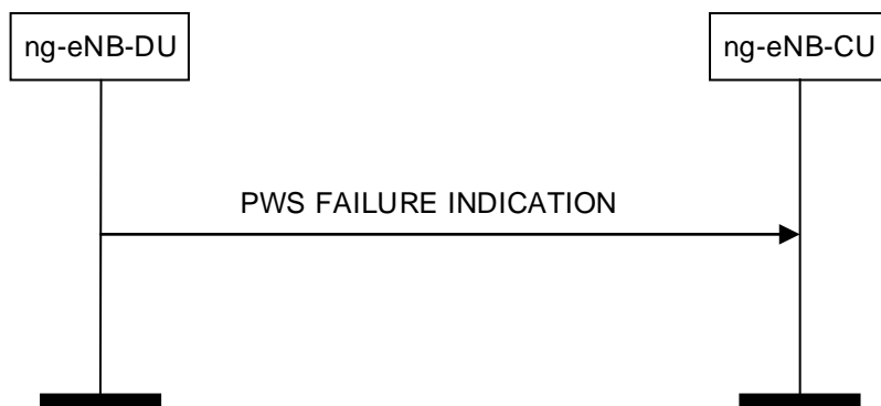
Figure 8.5.4.2-1: PWS failure indication
