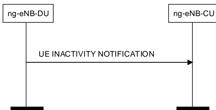
Figure 8.3.6.2-1: UE Inactivity Notification procedure.
