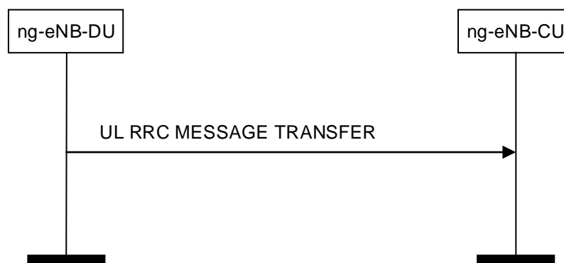
Figure 8.4.3.2-1: UL RRC Message Transfer procedure
