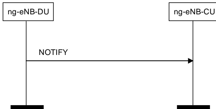
Figure 8.3.7.2-1: Notify procedure. Successful operation.
