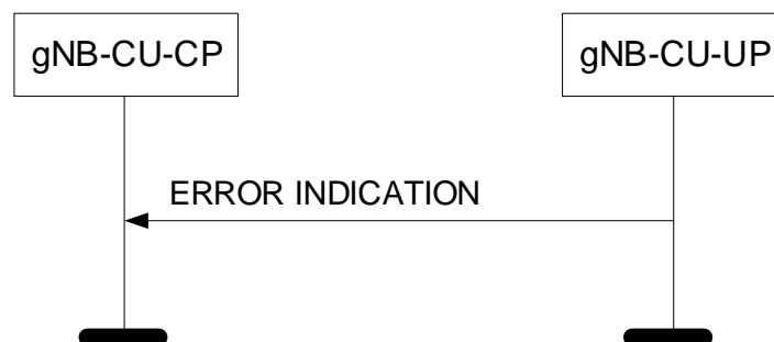
Figure 8.2.2.2-2: Error Indication procedure, gNB-CU-UP originated. Successful operation.
