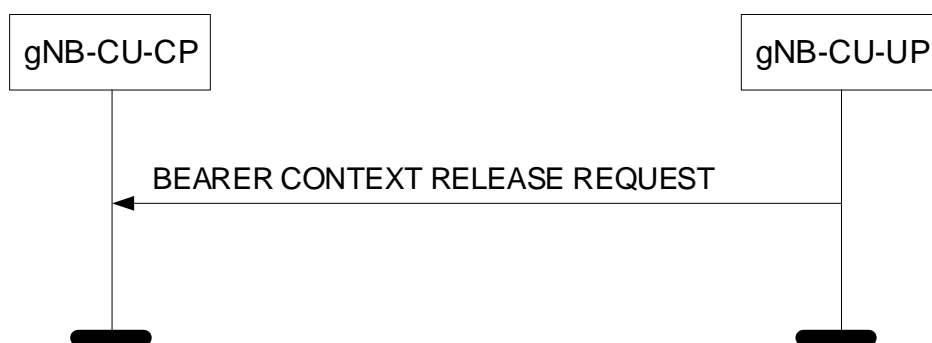
Figure 8.3.5.2-1: Bearer Context Release Request procedure: Successful Operation.
