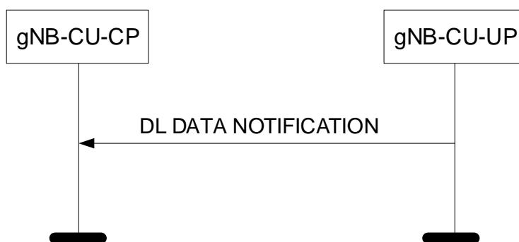
Figure 8.3.7.2-1: DL Data Notification procedure: Successful Operation.
