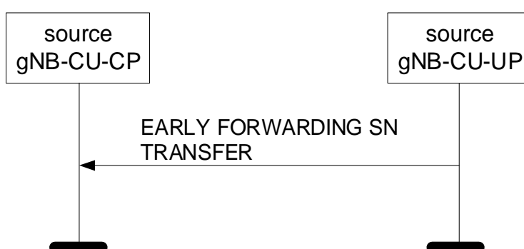
Figure 8.3.12.2-1: Early Forwarding SN Transfer procedure: Successful Operation.
