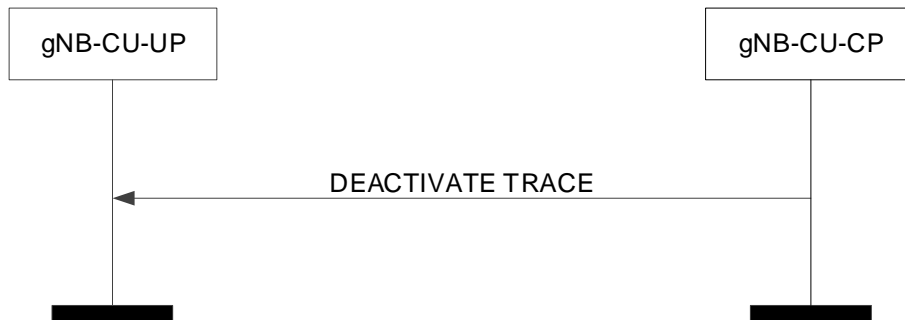
Figure 8.4.2.2-1: Deactivate trace procedure: Successful Operation.
