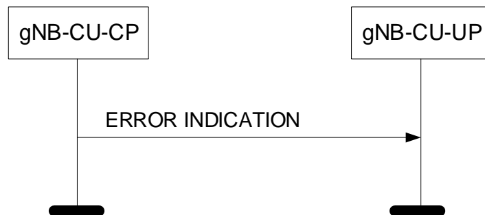
Figure 8.2.2.2-1: Error Indication procedure, gNB-CU-CP originated. Successful operation.
