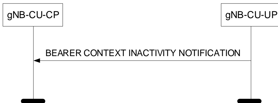
Figure 8.3.6.2-1: Bearer Context Inactivity Notification procedure: Successful Operation.
