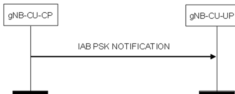
Figure 8.5.2.2-1: IAB PSK Notification procedure: Successful Operation.
