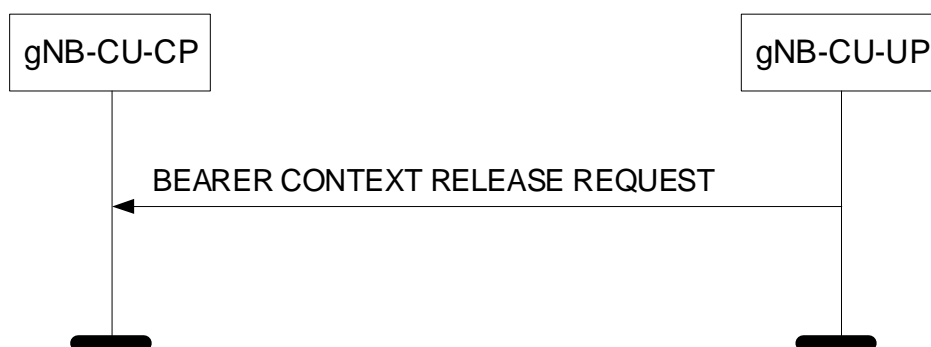
Figure 8.3.5.2-1: Bearer Context Release Request procedure: Successful Operation.
