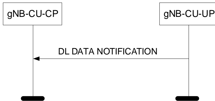
Figure 8.3.7.2-1: DL Data Notification procedure: Successful Operation.
