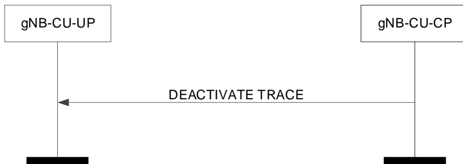
Figure 8.4.2.2-1: Deactivate trace procedure: Successful Operation.
