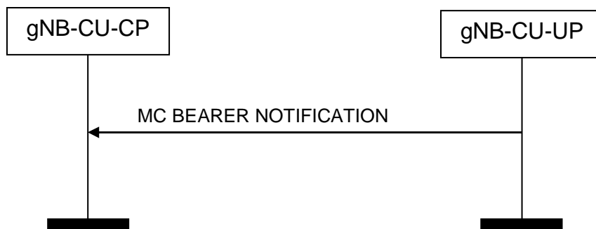
Figure 8.6.2.6.2-1: MC Bearer Notification procedure: Successful Operation.
