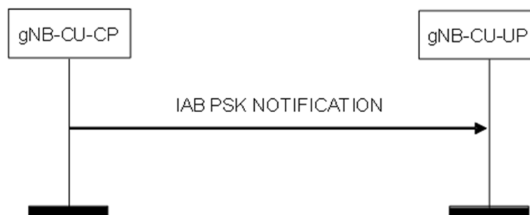
Figure 8.5.2.2-1: IAB PSK Notification procedure: Successful Operation.
