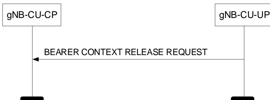
Figure 8.3.5.2-1: Bearer Context Release Request procedure: Successful Operation.
