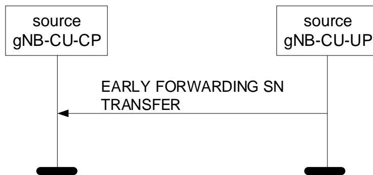
Figure 8.3.12.2-1: Early Forwarding SN Transfer procedure: Successful Operation.
