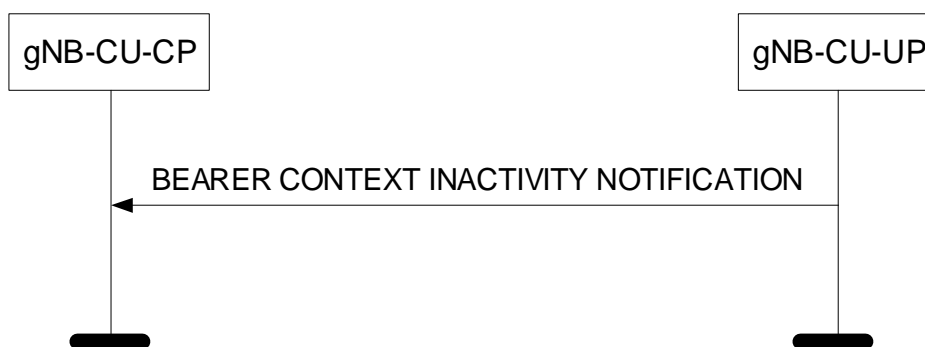
Figure 8.3.6.2-1: Bearer Context Inactivity Notification procedure: Successful Operation.
