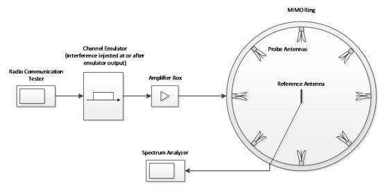
Figure B.2.3.1-2: Example setup for step 2 of the calibration
