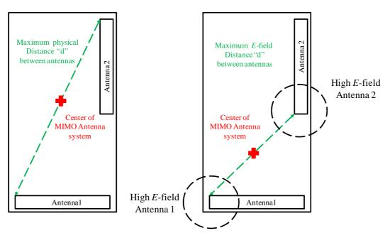
Figure A.5.2.1-2: Definition of distance between MIMO antennas and DUT center, maximum physical separation, or E-field maximum separation defined by manufacturer
