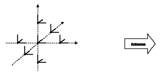
Figure G.2.1-1: Measurement positions with 150mm separation
