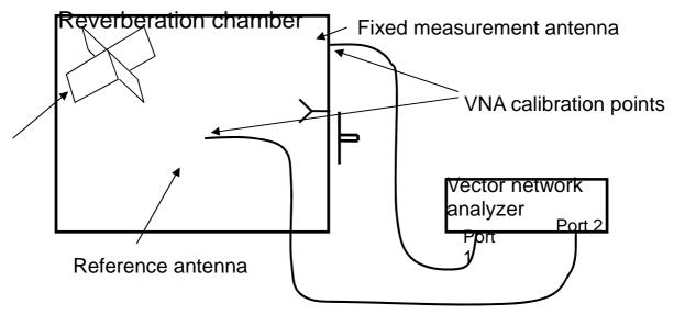
Figure B.2.2-1: Calibration measurement setup in the reverberation chamber, using a vector network analyzer
