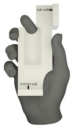
Figure 4.3.3.4-1: Right-handed PDA hand phantom with a spacer
