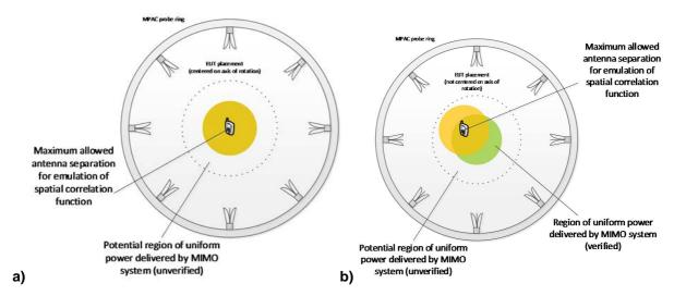
Figure A.5.2.1-1: Illustration of DUT antenna spacing and positioning guidelines; a) guideline in this specification, b) example with DUT meeting the maximum allowed antenna separation but not within the verified power stability region
