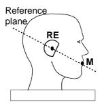
Figure 4.3.1-2: Reference plane on head phantom, side view
