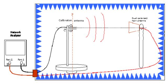
Figure B.2.1-1: Calibration/substitution procedures using a vector network analyzer
