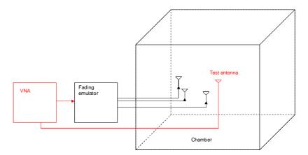
Figure B.2.3.1-1: Setup for VNA measurements
