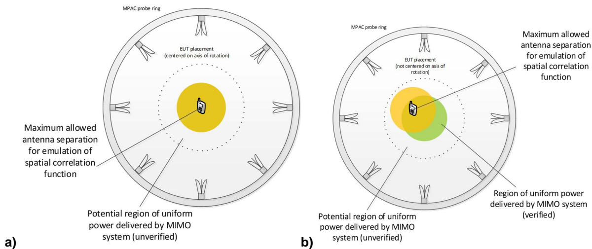
Figure A.5.2.1-1: Illustration of DUT antenna spacing and positioning guidelines; a) guideline in this specification, b) example with DUT meeting the maximum allowed antenna separation but not within the verified power stability region
