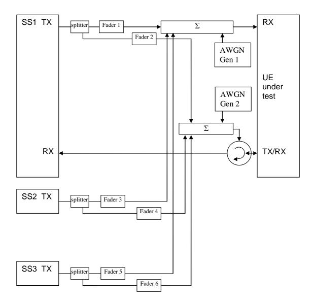
Figure A.4: Connection for 3 cells OTDOA tests with multipath fading propagation conditions
