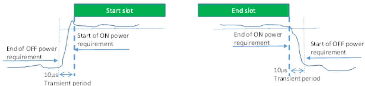
Figure 6.3.3.2-1: General ON/OFF time mask for NR UL transmission in FR1
