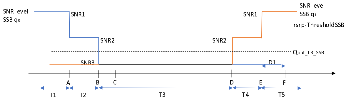
Figure A.7.5.5.1-1: SNR variation SSB for SSB-based beam failure detection and link recovery testing in non-DRX mode
