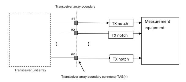
Figure D.3.3-2: Measuring system set-up for transmitter spurious emissions for multiple *TAB* connectors in parallel test
