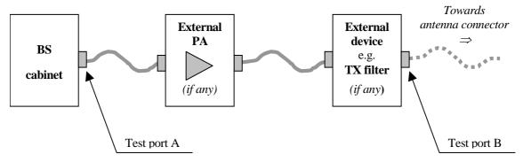
Figure 4.5.1.1.1-1: Transmitter test ports
