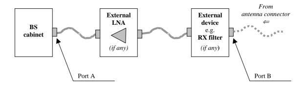
Figure 4.2.1-2: BS type 1-C receiver interface
