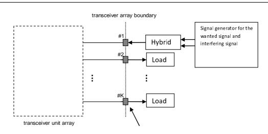
Figure D.4.5-1: Measuring system set-up for BS type 1-H in-channel selectivity test
