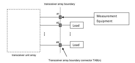
Figure 4.5.2.2-1: Receiver test ports
