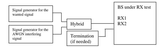
Figure D.2.2-1: Measuring system set-up for BS type 1-C dynamic range
