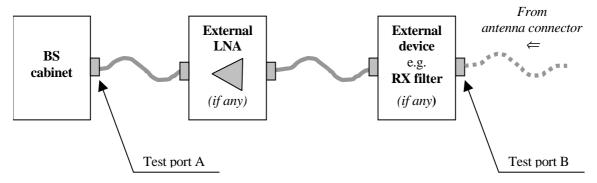
Figure 4.5.1.2.1-1: Receiver test ports
