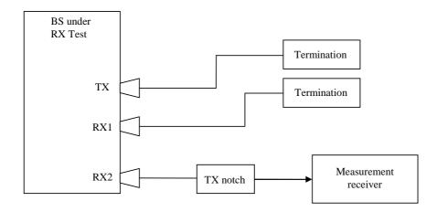
Figure D.2.6-1: Measuring system set-up for BS type 1-C receiver spurious emission
