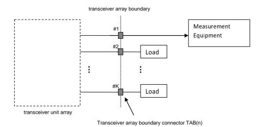
Figure 4.5.2.1-1: Transmitter test ports
