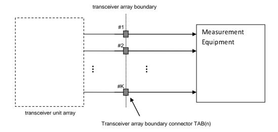
Figure D.3.1-2: Measuring system set-up for BS type 1-H output power, output power dynamics, transmitter ON/OFF power, frequency error, EVM, unwanted emissions for multiple TAB connectors
