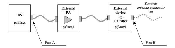
Figure 4.2.1-1: BS type 1-C transmitter interface
