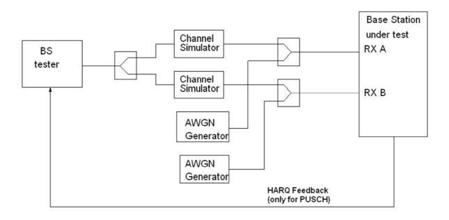
Figure D.5.1-1: Functional set-up for performance requirements for PUSCH, single user PUCCH, PRACH on single antenna port in multipath fading conditions for BS with Rx diversity (2 Rx case shown)
