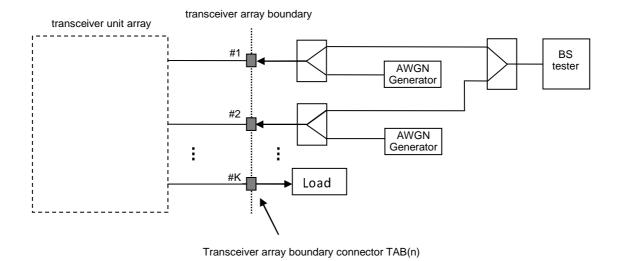
Figure D.6.3-1: Functional set-up for performance requirements for PRACH in static conditions for BS with Rx diversity (2 Rx case shown)
