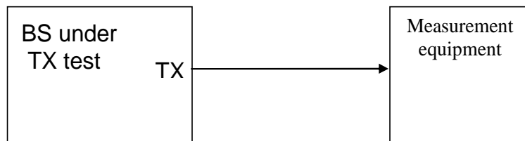
Figure D.1.1-1: Measuring system set-up for BS type 1-C output power, output power dynamics, frequency error, EVM, unwanted emissions
