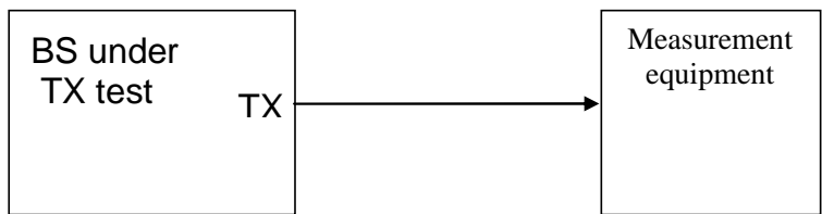
Figure D.1.1-1: Measuring system set-up for BS type 1-C output power, output power dynamics, frequency error, EVM, unwanted emissions
