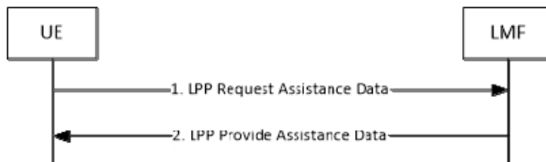
Figure 8.11.3.1.2.2-1: UE-initiated Assistance Data Transfer Procedure
