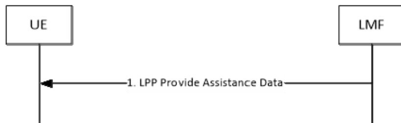
Figure 8.11.3.1.2.1-1: LMF-initiated Assistance Data Delivery Procedure
