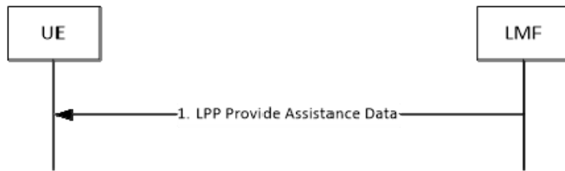
Figure 8.10.3.1.2.1.1-1: LMF-initiated Assistance Data Delivery Procedure
