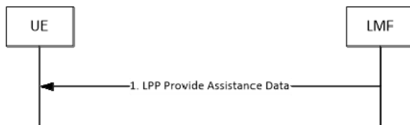
Figure 8.11.3.1.2.1-1: LMF-initiated Assistance Data Delivery Procedure
