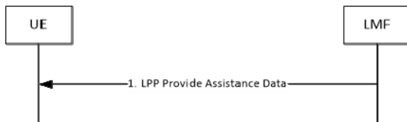
Figure 8.10.3.1.2.1.1-1: LMF-initiated Assistance Data Delivery Procedure
