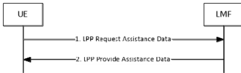
Figure 8.11.3.1.2.2-1: UE-initiated Assistance Data Transfer Procedure
