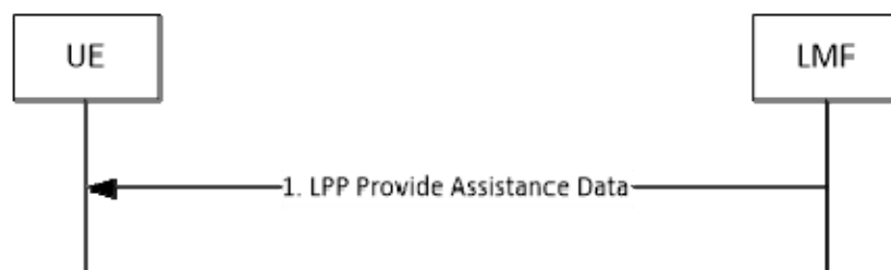
Figure 8.11.3.1.2.1-1: LMF-initiated Assistance Data Delivery Procedure
