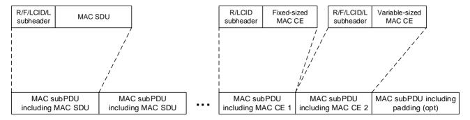
Figure 6.1.2-5: Example of a UL MAC PDU
