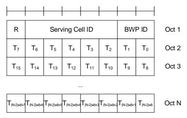
Figure 6.1.3.14-1: TCI States Activation/Deactivation for UE-specific PDSCH MAC CE
