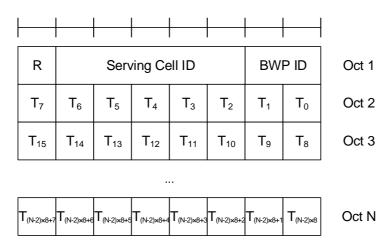
Figure 6.1.3.13-1: Aperiodic CSI Trigger State Subselection MAC CE
