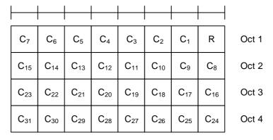
Figure 6.1.3.10-2: SCell Activation/Deactivation MAC CE of four octets
