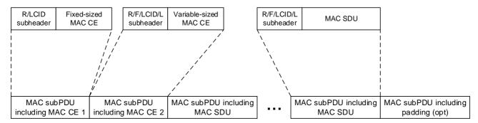
Figure 6.1.2-4: Example of a DL MAC PDU
