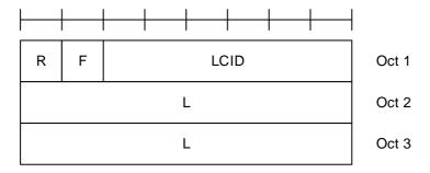
Figure 6.1.2-2: R/F/LCID/L MAC subheader with 16-bit L field
