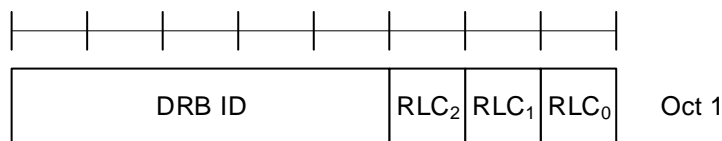
Figure 6.1.3.32-1: Duplication RLC Activation/Deactivation MAC CE
