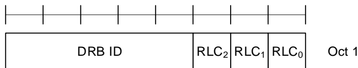
Figure 6.1.3.32-1: Duplication RLC Activation/Deactivation MAC CE
