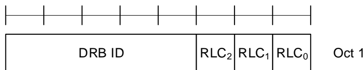
Figure 6.1.3.32-1: Duplication RLC Activation/Deactivation MAC CE
