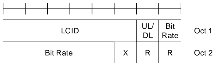
Figure 6.1.3.20-1: Recommended bit rate MAC CE
