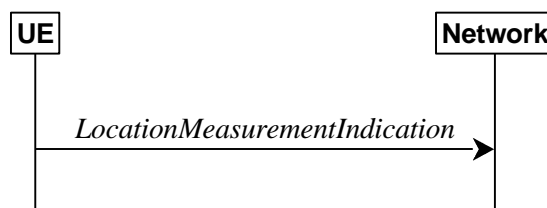
Figure 5.5.5.1-1: Location measurement indication
